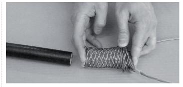
Press the Hoisting Grip to allow insert on cable.
