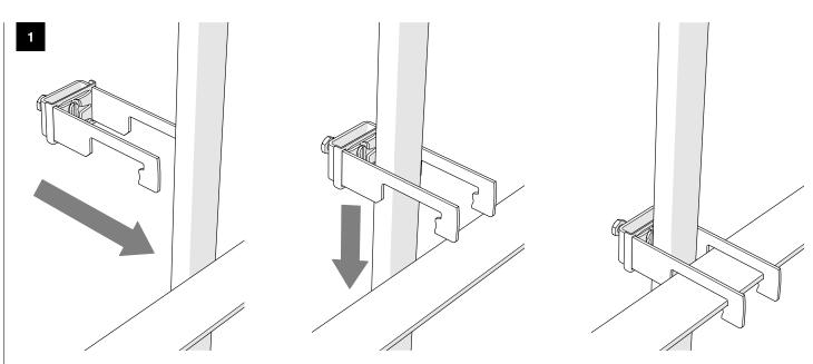
1 - Place the bow around the cables and hook it on the support.
