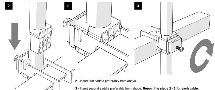
4 - Tighten self-locking screw 1-2 Nm.
