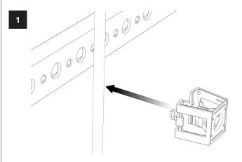
Insert Sic Snap-In clamp on the cable.
