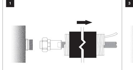
Slip in the cold shrink tube before connection. Then connect the  $1/2^{\circ}$  jumper to antenna.
