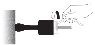
Counterclockwise rotate and pull out the plastic core, the tube will shrink.
