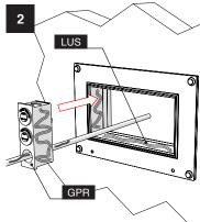
Remove the temporary protection film. Carefully lubricate the inside wall entry surfaces by LUS lubricant. Lubricate inside and outside the GPR cushions and insert them onto the cables.
