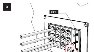
Tighten progressively and alternatively the 3 screws of the expander GPE. Max tightening torque = 4 Nm.
