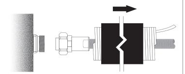
Slip in the cold shrink tube before connection. Then connect the 1/2" jumper to antenna.
