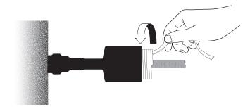
Counterclockwise rotate and pull out the plastic core, the tube will shrink.
