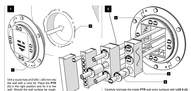
wall. Should the wall surface be rough, put some BUT 6 (2) butilic putty or some silicone grease between wall and PTR.
