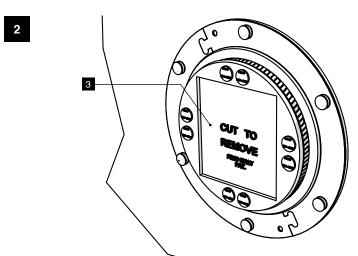
Remove the temporary protection sheet (3).
