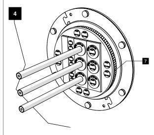
For the final sealing, tightly lock the stainless steel hose clamp (7).
