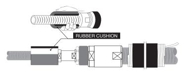
Remove the protective film around rubber cushion. Remove protective film from butyl tape connecting two halves of round cushion. Apply round cushion around jumper cable, closing the two halves together.
