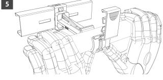
Insert cable into RAX clamp contrasting from below.
