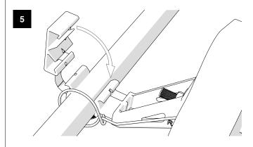
Close **RSD** around the cable\*, place **RAW** outer bracket end
