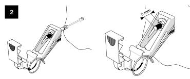
Insert the **MF/MFI** anchor in the hole with the **RAW** clamp, leaving 5mm prominent from nut. If necessary use a hammer to facilitate insertion
