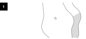
Drill a Ø 6-8mm hole in accordance with anchor MF/MFI Ø - Clean the hole
