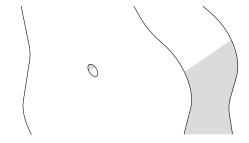
**Drill a \emptyset 8-10mm hole** in accordance with plug  $\emptyset$  - Clean the hole
