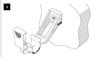
Tighten the screw (4-5 Nm) for complete lock
