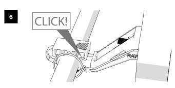
Close **RAW** bracket over cable with a **CLICK!** at inner end
