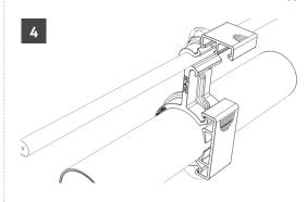
Insert rope into smaller RAR housing.
