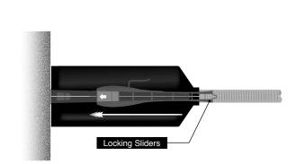
Slide in the Locking Slider. You will hear a "CLICK" sound when fitted properly.
