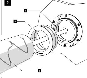
Carefully lubricate the inside PTR wall entry surfaces with LUS 8 silicone grease (4). Spread some LUS 8 on both the inner and outer surfaces of the GRR (5) round reduction cushion; lubricate the cable externally (6). Insert the GRR reduction cushion in the PTR wall entry, insert the cable in the GRR round reduction cushion and carefully place it inside the PTR wall entry.
