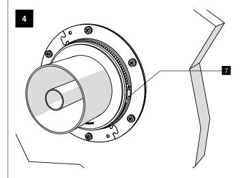
For the final sealing, tightly lock the stainless steel hose clamp (7).
