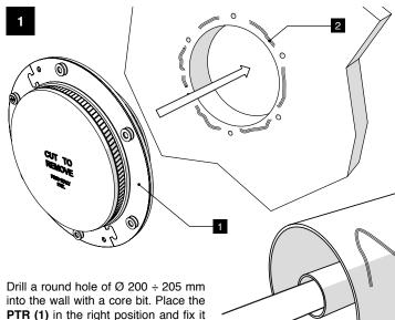
Drill a round hole of Ø 200 ÷ 205 mm into the wall with a core bit. Place the PTR (1) in the right position and fix it to the wall. Should the wall surface be rough, put some BUT 6 (2) butilic putty or some silicone grease between wall and PTR.
