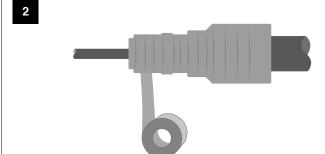
Wrap the connection with a layer of 19 mm plastic adhesive tape.
