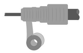
Wrap two layers of 50 mm adhesive plastic tape overlapping at half width.
