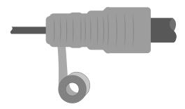
Wrap three layers of 19 mm adhesive plastic tape overlapping at half width.
