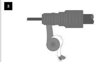
Expand the width of the 50 mm butyl tape by stretching it so that it will wrap completely around the connector and cable. Wrap the butyl tape around the cable and the connector cable.
