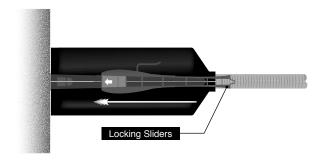
Slide in the Locking Slider. You will hear a "CLICK" sound when fitted properly.
