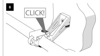
Close RAW bracket over cable with a CLICK! at inner end
