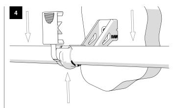
Insert cable into **RAW** clamp contrasting from below
