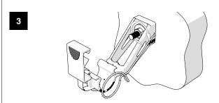
Tighten the nut (4-5 Nm) for complete lock
