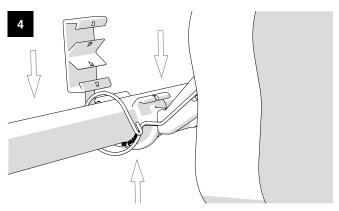
Insert cable into **RSD** security device\*, and then insert cable into **RAW** clamp contrasting from below
