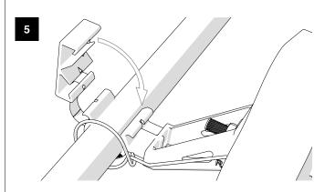
Close **RSD** around the cable\*, place **RAW** outer bracket end
