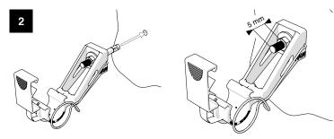
Insert the **MF/MFI** anchor in the hole with the **RAW** clamp, leaving 5mm prominent from nut. If necessary use a hammer to facilitate insertion
